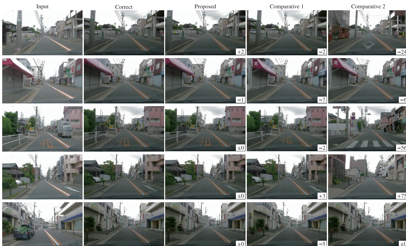
Fig. 8. Search result of Sequence 5 from Sequence 3. The value in the bottom right of each image shows the difference (number of frames) from the correct corresponding image.
