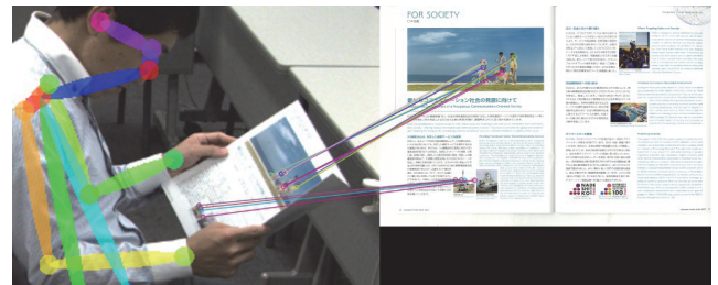
Fig. 4 Keypoint matching to find the reading page
