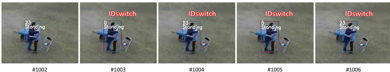
Fig. 9: Example of frequent ID switches because two humans are detected in only one bounding box alternately.
