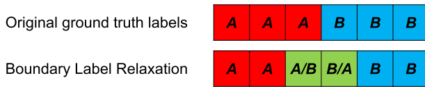
Fig. 1. Boundary Label Relaxation (BLR) in 1D label space. The ground truth of the border pixels (shown in green) are modified to contain class labels that appear in both sides of the border. (For interpretation of the references to colour in this figure legend, the reader is referred to the web version of this article.)
