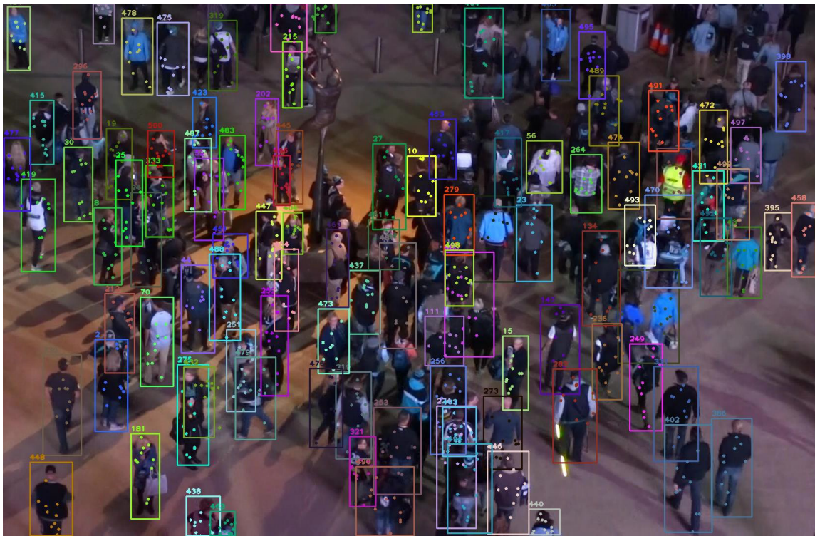
Fig. 5 Example of tracking result using the SDOF-Tracker with SCT.
